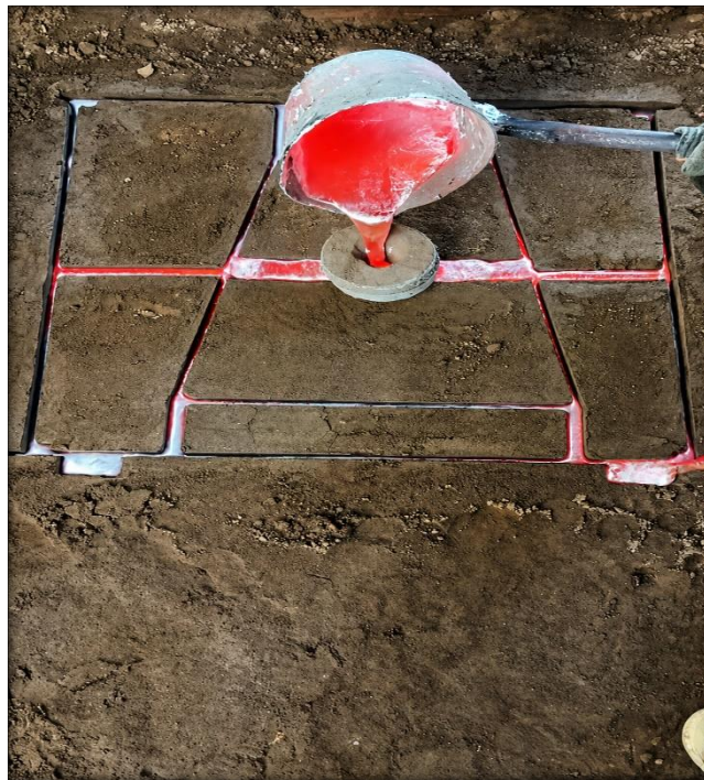
Fig 4: Pouring of molten aluminium into mould (Fieldwork, 2026)
