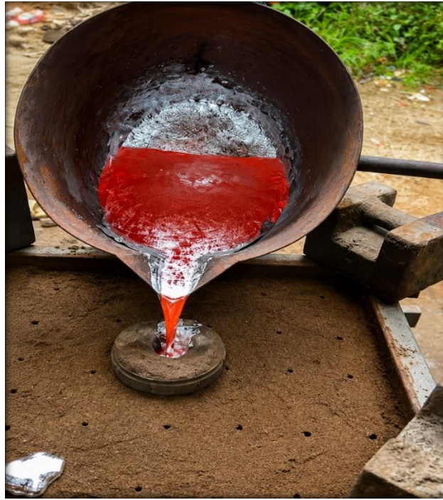
Fig 2: Simpler furnaces with metal crucible for molten aluminium (Fieldwork, 2026)
