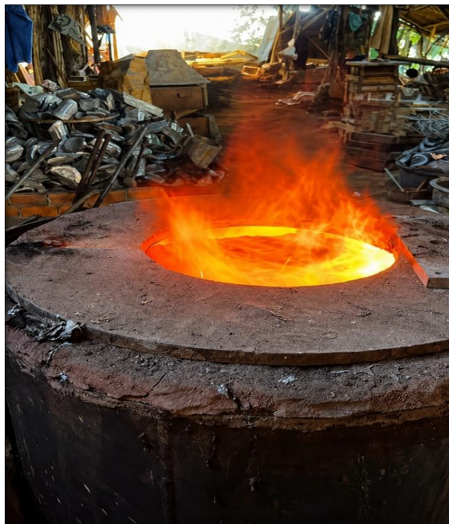
Fig 3: Melting aluminium for casting (Fieldwork, 2026)
