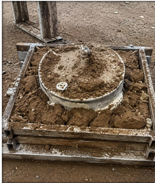
Fig 5: Breaking apart the mould to reveal cast piece (Fieldwork, 2026)
