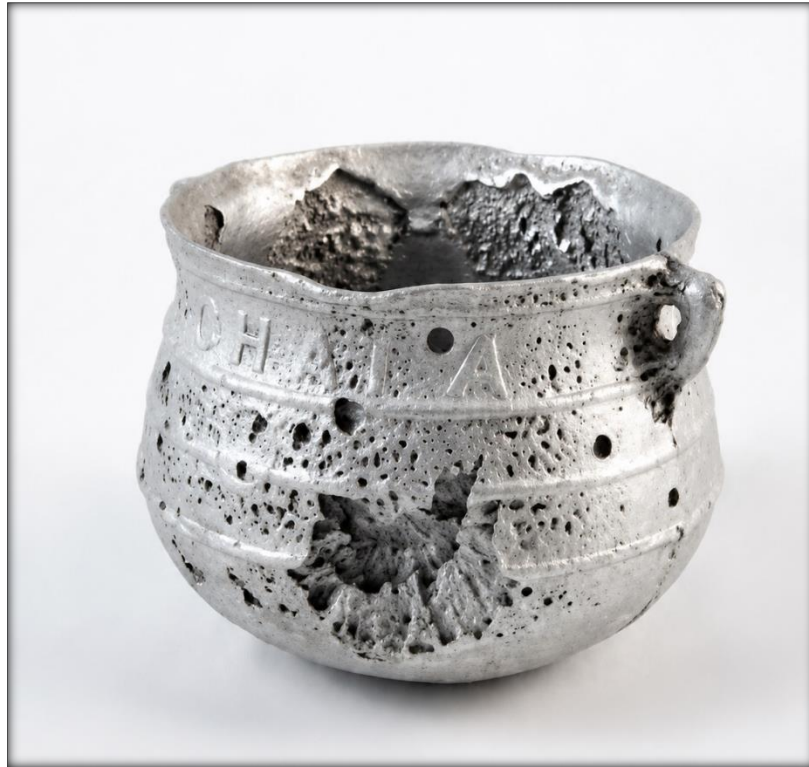
Fig 6: Various defects in cast piece (Fieldwork, 2026)
